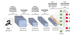
Fig. 8. Working of Convolution Neural Network
