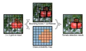
Fig. 2. YOLO Object Detection
